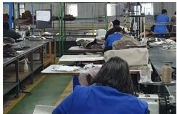
Example of a sewing line with live performance display at the front of the line
